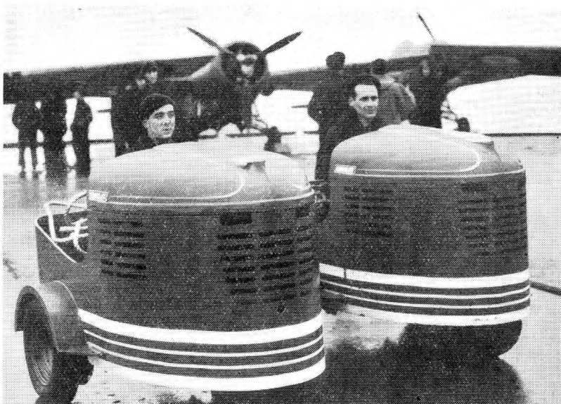
These tractors, known as dodgem s, are used for pulling aircraft about on the flight deck of a carrier.
