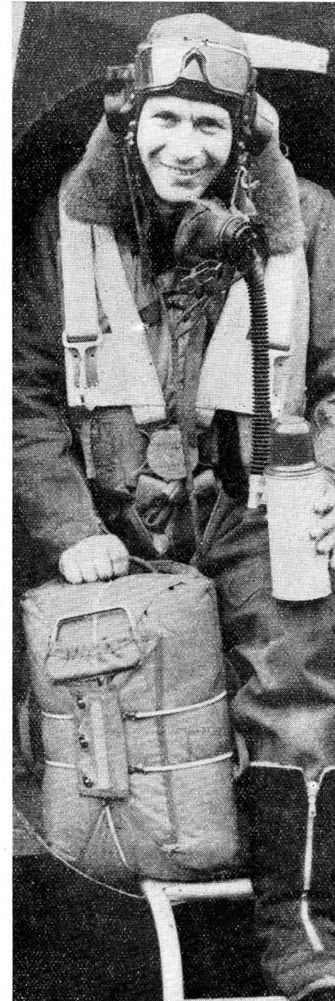
This picture of Sergeant L. R. Tonkin, an Australian, leaving a Stirling, presents a good view of the observer-type parachute pack and harness.
