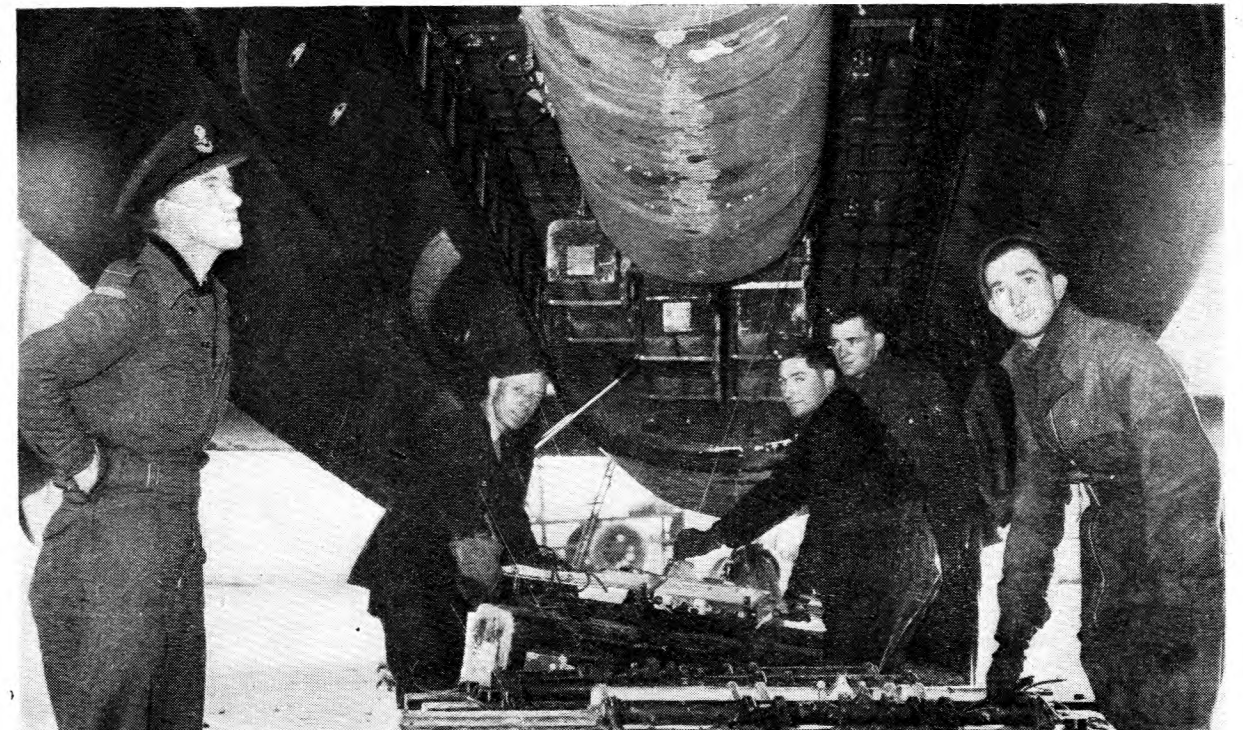
Loading up a case of incendiaries alongside a blockbuster on a Lancaster.
