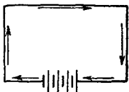
Figs. 2 and 3.—Diagrams showing the movement of electrons in a D.C. and an A.C. circuit.
