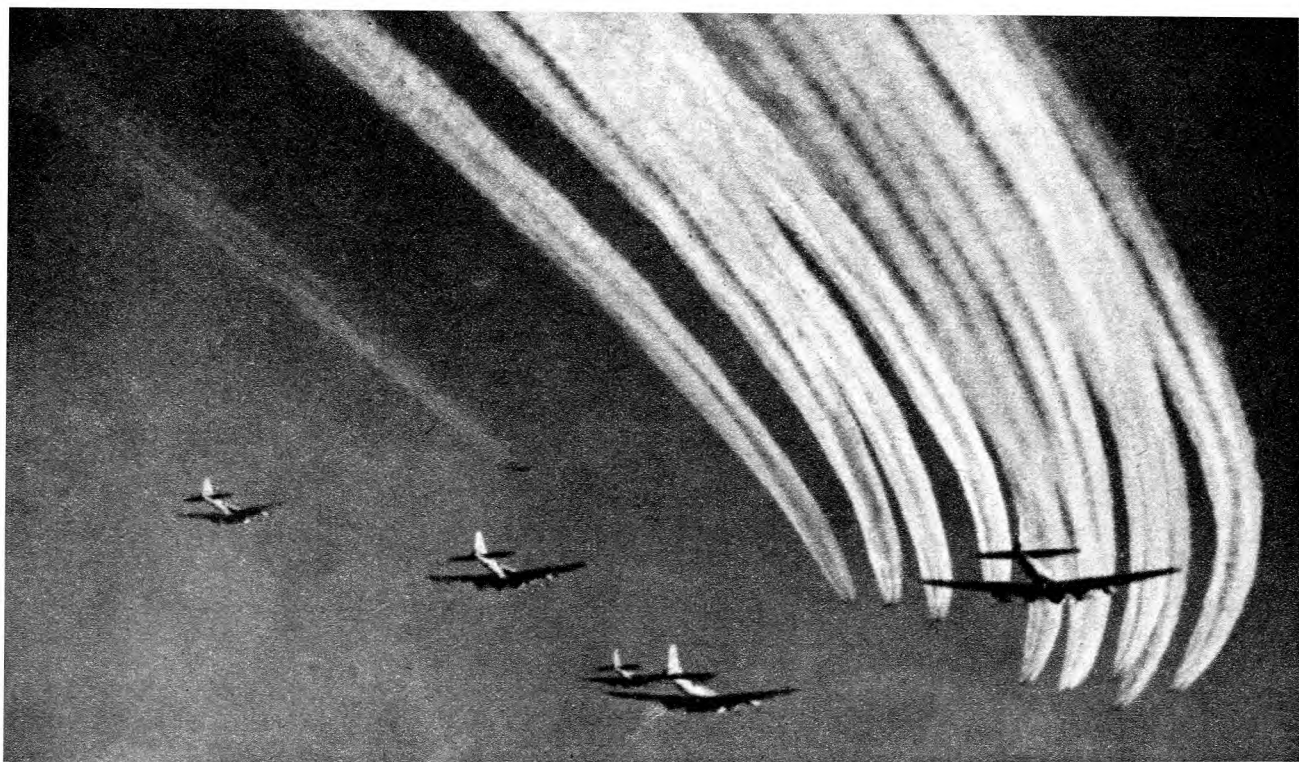
Vapor trails at 25,000. Condensation in the upper altitudes often leaves a white trail behind each plane.
